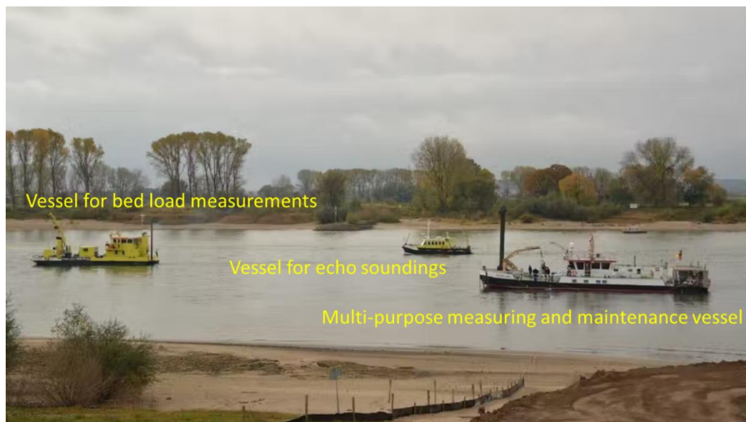
Figure 18 Boats equipped with equipment for measuring sediment transport, soundings and tools for regular maintenance work (Rhine River at Lobith, border between Germany and The Netherlands).
